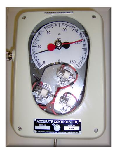
Configured as an Oil Temperature Indicator (OTI) or Winding Temperature Indicator (WTI) for simulation of transformer 'Hot Spot' temperature.
